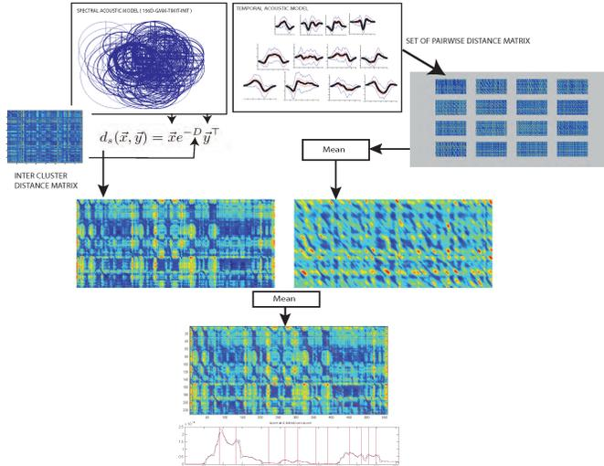
**Fig. 1.** Schematics of the system. Two acoustic models generate pairwise distances between query and reference. The matrices are fused into a single matrix where alignment paths are searched and filtered.
